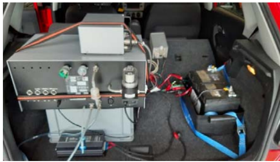
Figure 2-4: Automotive 5-gas tester, 12V battery, 12/24 V DC-converter, pressure sensor box for a pitot tube and SEMS data logger in the trunk.
